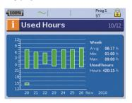
Used Hours during the last seven days of treatment are displayed in a bar graph and can be compared to the data of the last 365 days.
