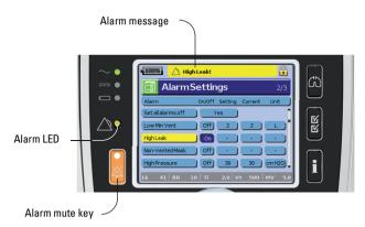
Alarm messages are displayed along the top of the screen. High priority alarms are displayed in **red**, medium priority alarms in **yellow** and low priority alarms in **light blue**. The Alarm LED lights **red** during high priority alarms and **yellow** during medium and low priority alarms
