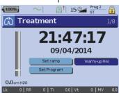
You can use the warm-up feature to pre-heat the water in the humidifier prior to starting treatment. The humidifier will be automatically detected when the device is turned on. The *Treatment* screen provides the option to start warming the humidifier. If the humidifier is heating, the related symbol is displayed at the top of the LCD screen.
