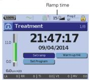
Ramp time is a feature that can be enabled by your clinician by setting a maximum ramp time. Designed to make the beginning of treatment more comfortable, ramp time is the period during which the pressure increases from a low start pressure to the treatment pressure. See "Setup menu: Options" on page 18.
