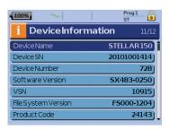
This screen shows the serial number (displayed as Device SN), device number, software version and other component versions. Data on this screen may be requested for servicing or as part of problem-solving by a technician.
