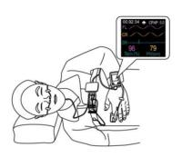
(3) Stop the recording by pressing and holding the **On-Off/OK Button** and **Shift Button** ①/⊙ + ⓒ simultaneously approximately three seconds. Power off device by pressing and holding **On-Off/OK Button** ①/⊙ for approximately five seconds.
